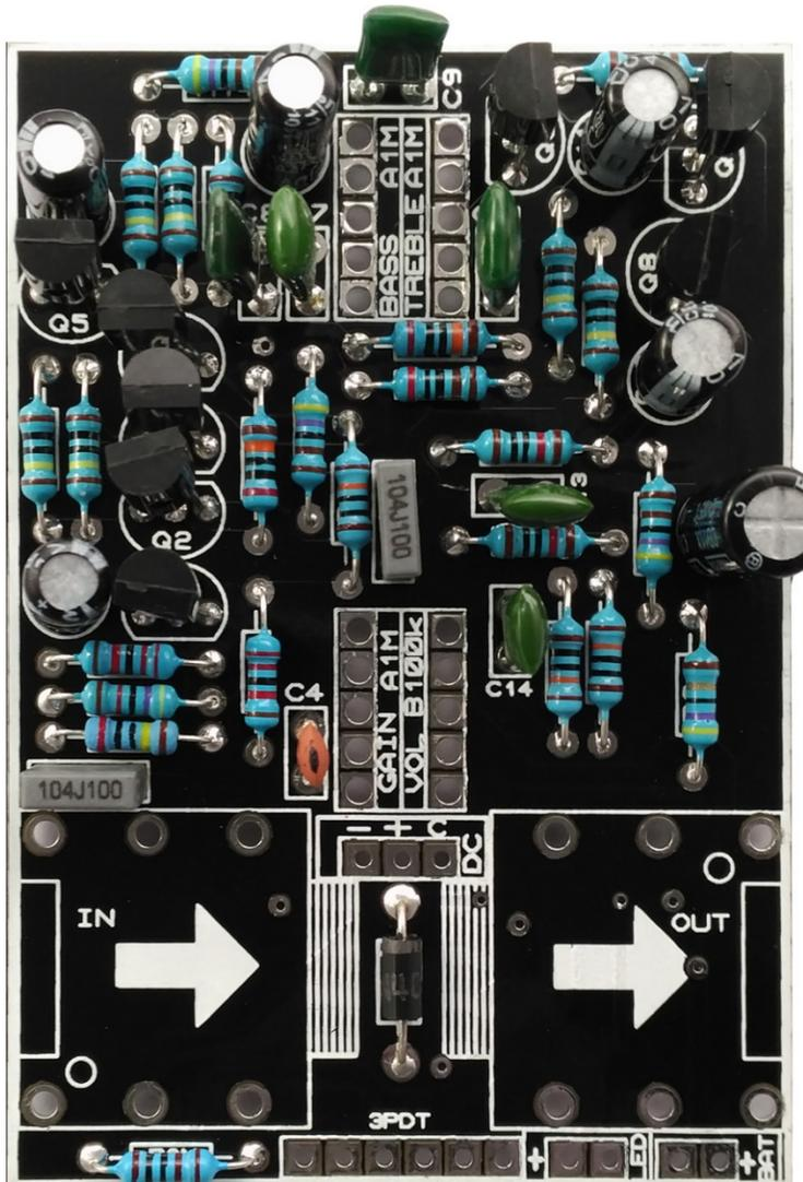
Solder the capacitors and transistors. If you have troubles reading the values, check out our [“Reading Part Values”](#) tutorial. Pay attention to the orientation, as well as to the polarity for electrolytic capacitors.
