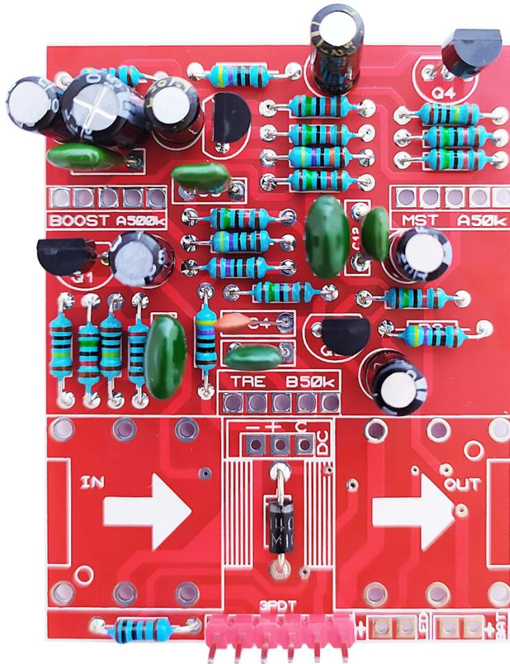
Solder the capacitors and transistors. If you have troubles reading the values, check out our [“Reading Part Values”](#) tutorial. Pay attention to the orientation, as well as to the polarity for electrolytic capacitors.
