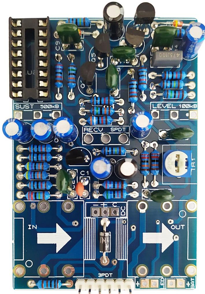
Solder the capacitors, transistors and the 2k trimmer. If you have troubles reading the values, check out our [“Reading Part Values”](#) tutorial. Pay attention to the orientation, as well as to the polarity for electrolytic capacitors.
