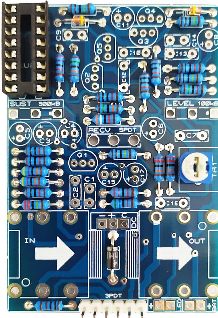
First of all place the IC socket (without the IC). Pay attention to the orientation! The small notch in the socket should be oriented as indicated in the PCB.
