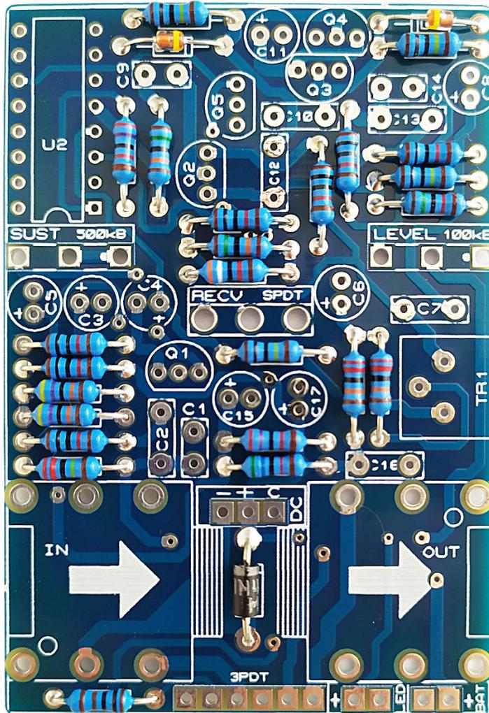
Place the resistors and diodes. If you have troubles reading the values, check out our ["Reading Part Values"](#) tutorial.
