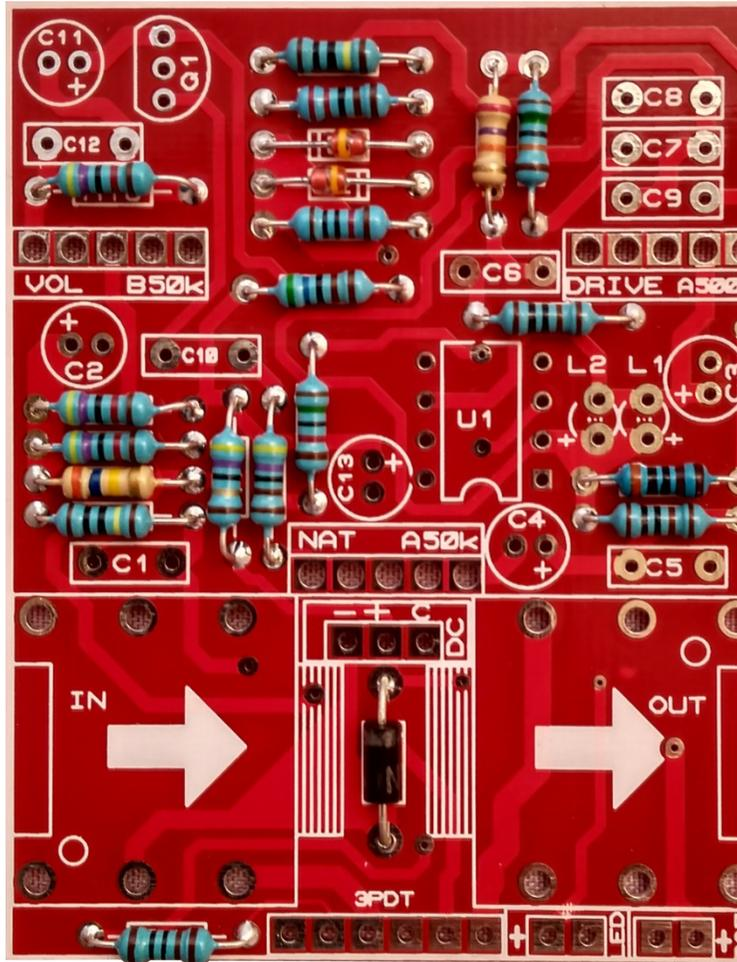
Place the resistors and diodes. If you have troubles reading the values, check out our ["Reading Part Values"](#) tutorial.
