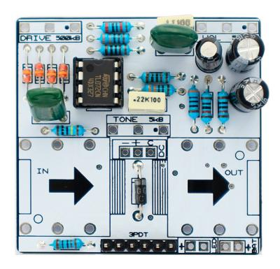
Solder the capacitors and transistors. If you have troubles reading the values, check out our <u>"Reading Part Values"</u> tutorial. Pay attention to the orientation, as well as to the polarity for electrolytic capacitors.
