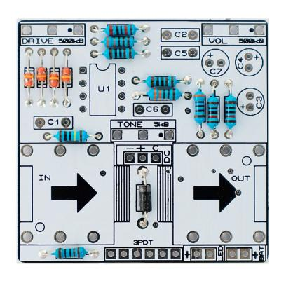
Place the resistors and diodes. If you have troubles reading the values, check out our "Reading Part Values" tutorial.
