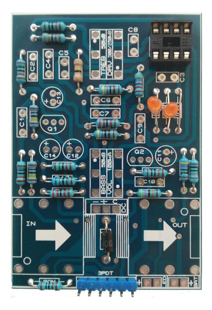
First of all place the IC sockets (without the ICs). Pay attention to the orientation! The small notch in the socket should be oriented as indicated in the PCB.
