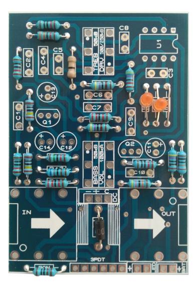
Place the resistors and diodes. If you have troubles reading the values, check out our <u>"Reading Part Values"</u> tutorial.
