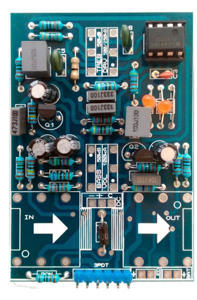
Solder the capacitors and transistors. If you have troubles reading the values, check out our <u>"Reading Part Values"</u> tutorial. Pay attention to the orientation, as well as to the polarity for electrolytic capacitors.
